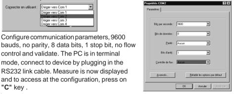
control and validate. The PC is in terminal mode, connect to device by plugging in the RS232 link cable. Measure is now displayed and to access at the configuration, press on "C" key . HyperTerminal
